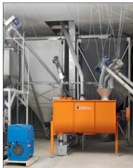
A horizontal mixer supplies the finished feed-mix to a HydroAir liquid feeding system
