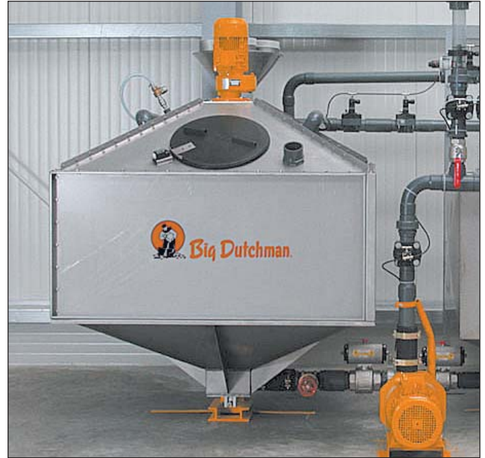
Stainless-steel feed mixing tank – large model
